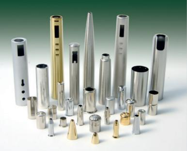
We produce deep-drawing parts with a length of up to 80 mm both on transfer presses and with follow-on composite tools. Besides steel and stainless steel strips also nonferrous metal is employed.
